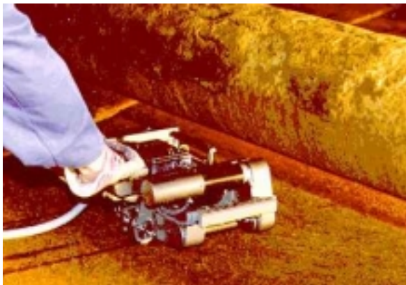
Fig. 7 Floor-scanner inspecting under-floor corrosion
